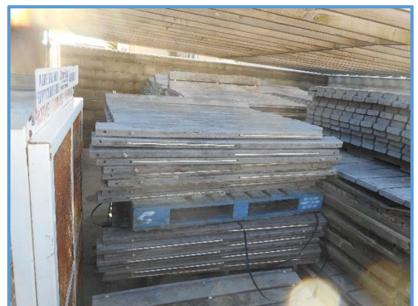
Rollout Composite Decking
